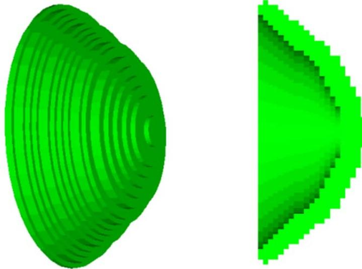
Figure 24. Fully formed copper penetrator, after 160  $\mu\text{s}$  (Autodyn) [8]
