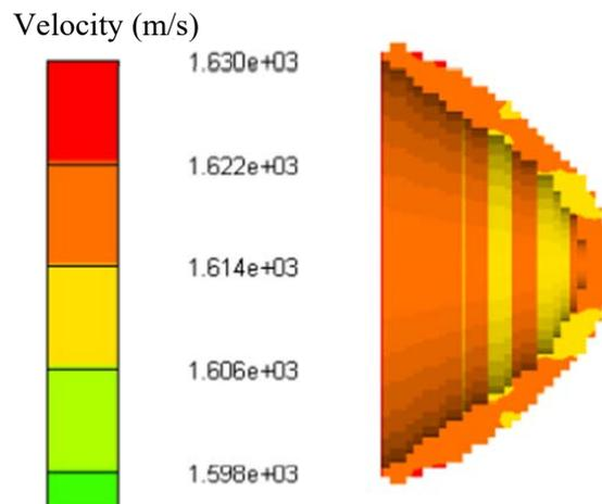
Figure 21. Velocity and shape of copper made penetrator (Autodyn); after 100  $\mu$ s – liner thickness is variable (2 mm – center; 1 mm – periphery) [8]
