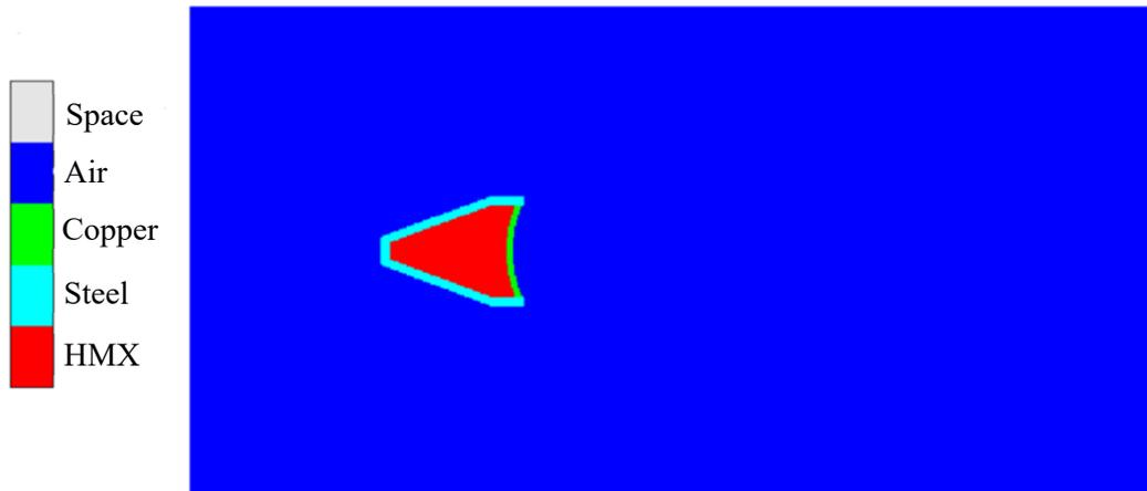
Figure 6. EFP model used in the research (Autodyn) [8]
