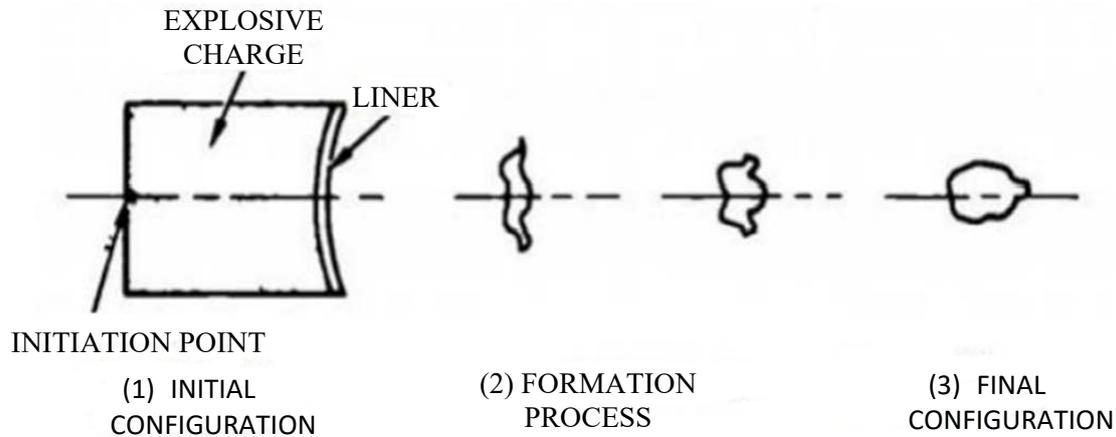
Figure 2. The formation process of EFP [3]
