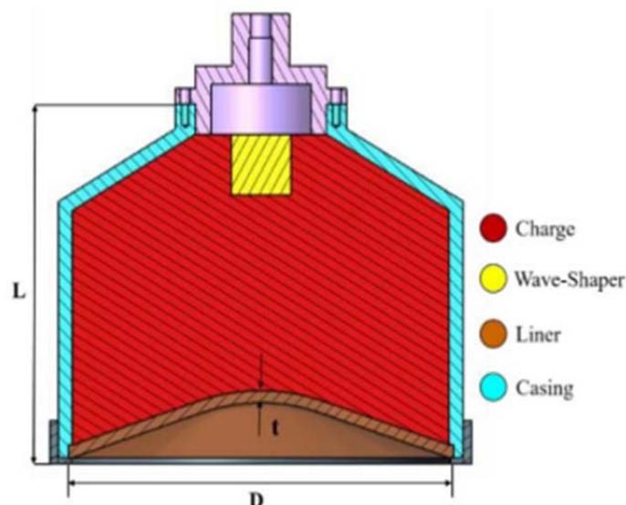
Figure 1. The schematic of EFP configuration [1]
