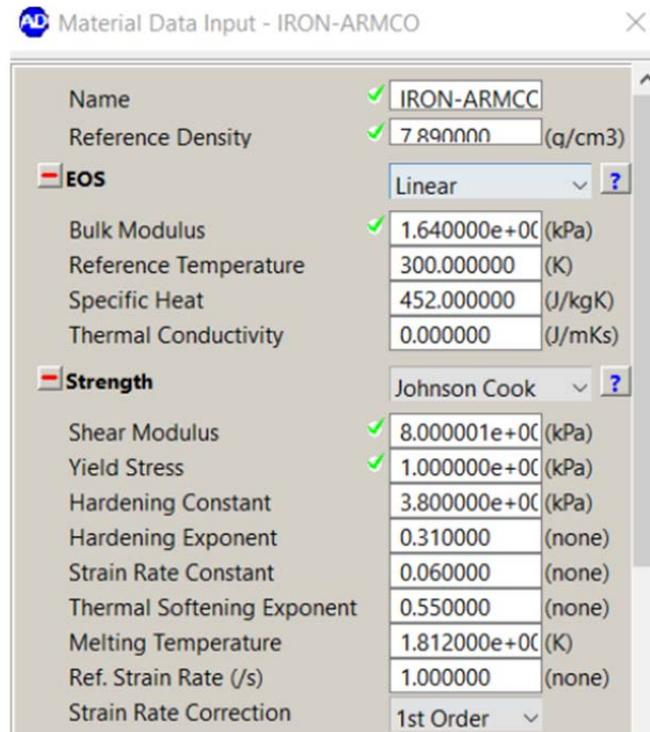
Figure 16. Characteristics of iron used in numerical simulation (Autodyn) [8]
