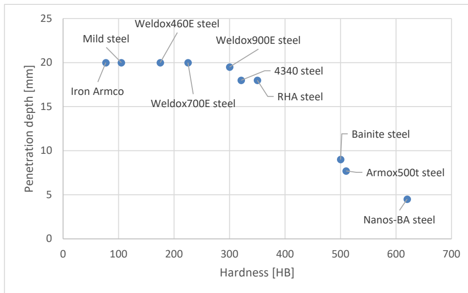
Figure 13. Diagram of penetration depth as a function of hardness
