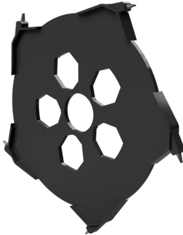
Figure 24. The most effective tiller shape for mine clearance
