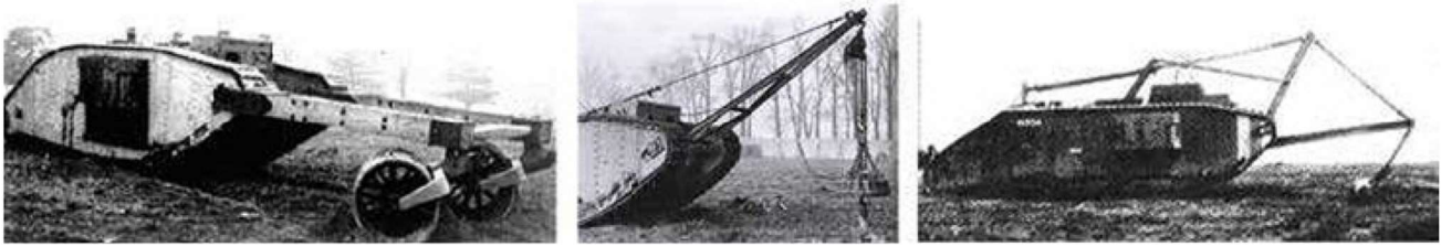
Figure 14. Early examples of mechanical demining, 1st World War, Mark IV tank that has been adapted for mine clearance
