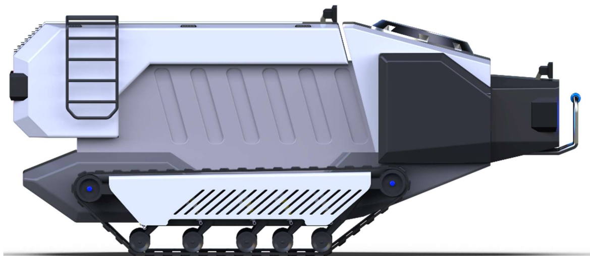
Figure 19. Side view of UGV modular platform with track-based power system
