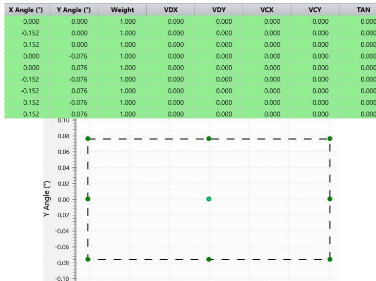
Fig. 16. Field points defined for JWST OTE model (represent rectangular FOV of 18' \times 9' )
