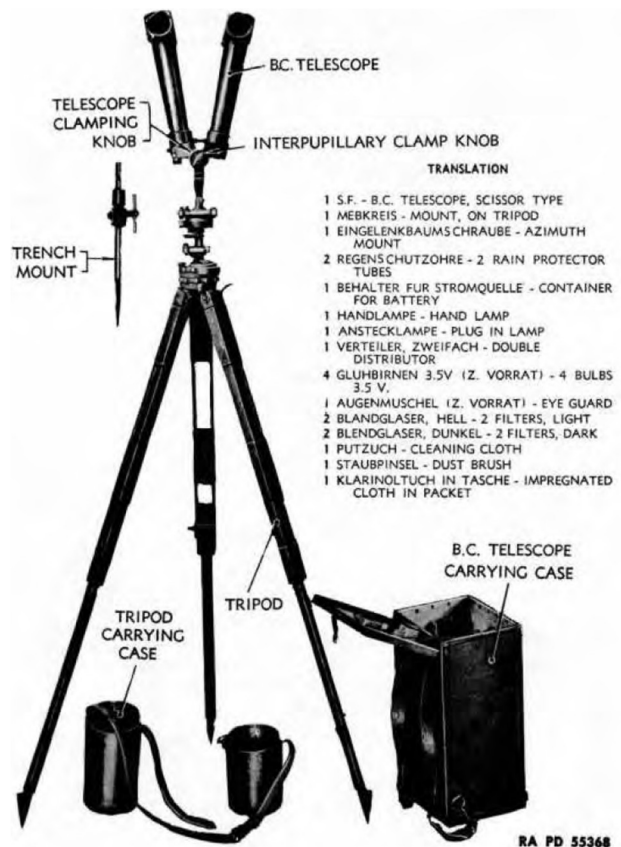
Fig. 18. Battery commander’s telescope with tripod and carrying cases [1]
