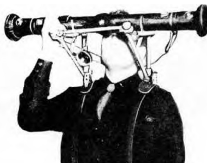
Fig. 15. Range finder 34 with shoulder harness in operational use [1]
