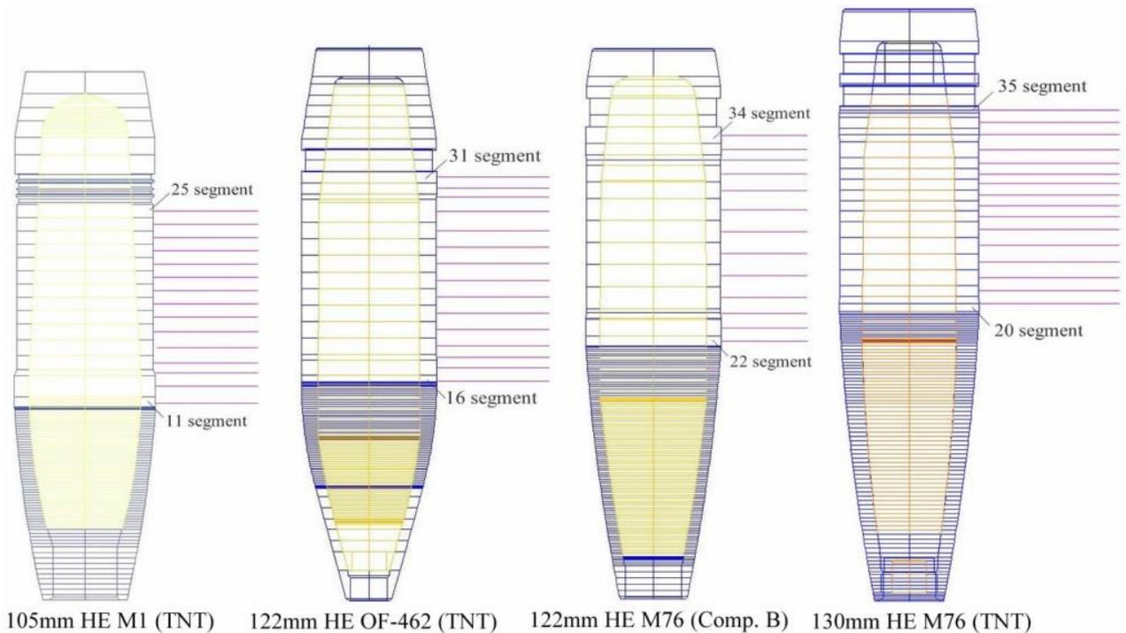
Figure 10. Body segments of artillery projectiles, for which Gurney method is applied, used in our model for determination of the lethal radius [20]
