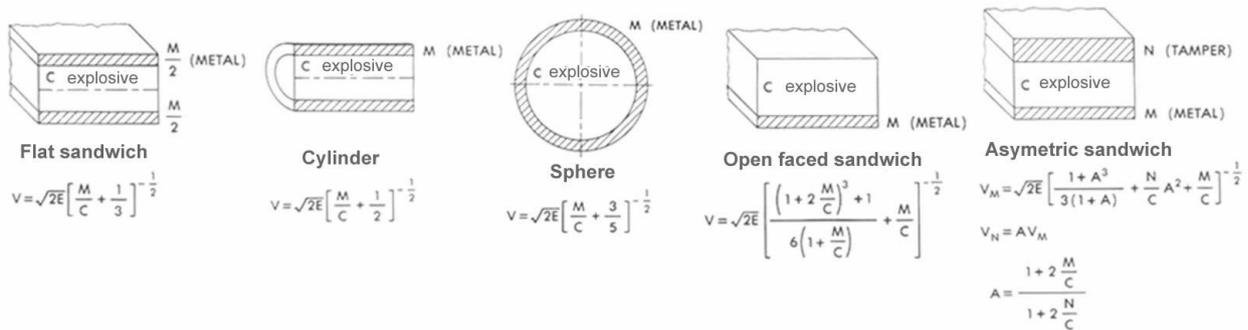
Fig. 2 Expressions for initial velocities of fragments in different geometric configurations [adopted from 2]
