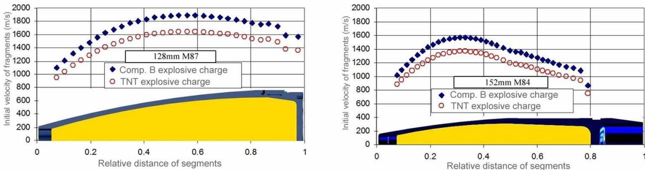
Figure 7. Variation of initial velocity of fragments, depending on the type of explosives (TNT and Composition B charge) for rocket projectile warhead - model 128mm HE M87 and artillery projectile - model 152mm HE M84 [19]
